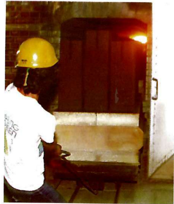
(Above) Refractory bricks are fired in a kiln at the Refractories Corporation of the Philippines.
